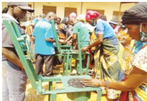
Participants moulding briquettes using the honeycomb manual machine during a training.
